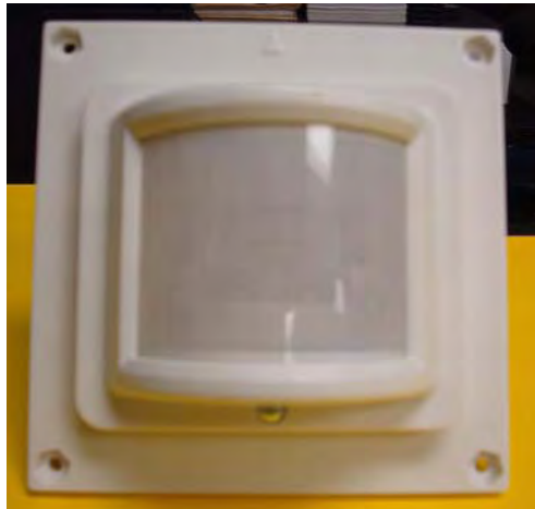
Figure 5. Assembled Flat 1.2" Lens Holder and Flat Lens
