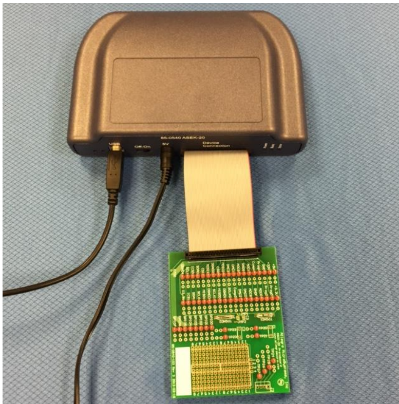
Figure 8: Photo shows ASEK-20 with USB cable, 5V power, ribbon cable and daughter board connected.
