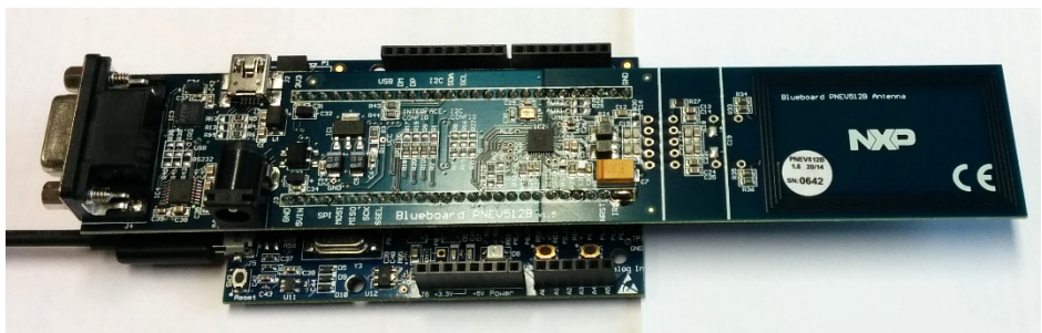
Fig 14. CLEV663B connected to LPCXpresso LPC11U68 development board
