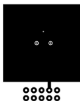
a. 74 °C/W when mounted on a 1 in 2 pad of 2 oz copper
