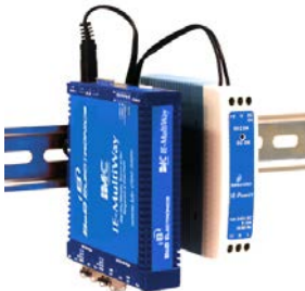
IE-MultiWay with optional DIN Rail mount power supply
