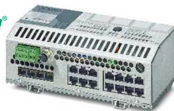
14 RJ45 ports and 2 FO ports
