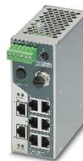
NAT switch with 8 RJ45 ports
