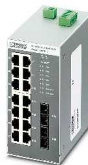
14 RJ45 ports and 2 FO ports
