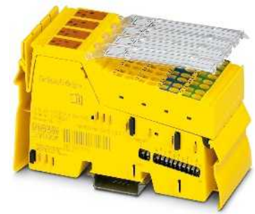
Connection of up to 16 safe input/output modules
