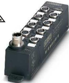
4 digital inputs and 4 digital outputs
