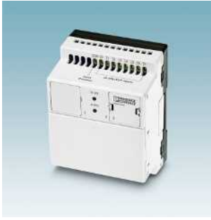
Nanoline – basic, extension, and communication modules
