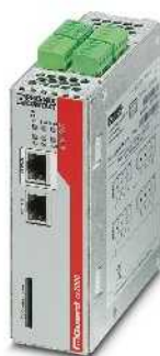
Router with simplified 2-click firewall and VPN
