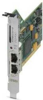
Router with firewall for PCI
