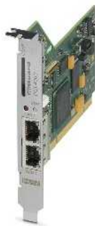
Router with firewall and VPN for PCI
