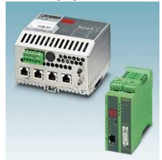
Proxies as a link between PROFINET networks and other fieldbus systems Page 326
