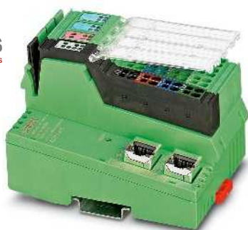
2-port RJ45 copper connection, 8 digital inputs and 4 digital outputs
