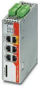
Router with intelligent firewall and integrated switch
