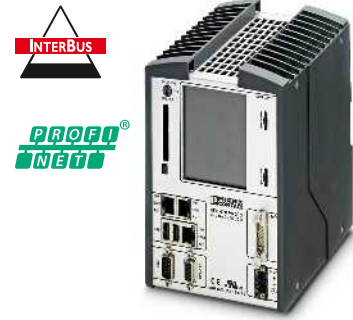
PLC, with optional integrated safety controller
