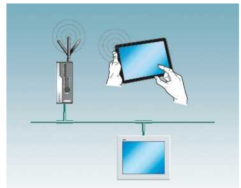
Visu+ mobile on a mobile terminal device via access point, with a touch panel and integrated web server
