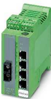
4 RJ45 ports and 1 fiber optic port (multi mode)
