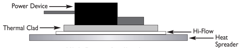
High Power Application Hi-Flow with Thermal Clad
